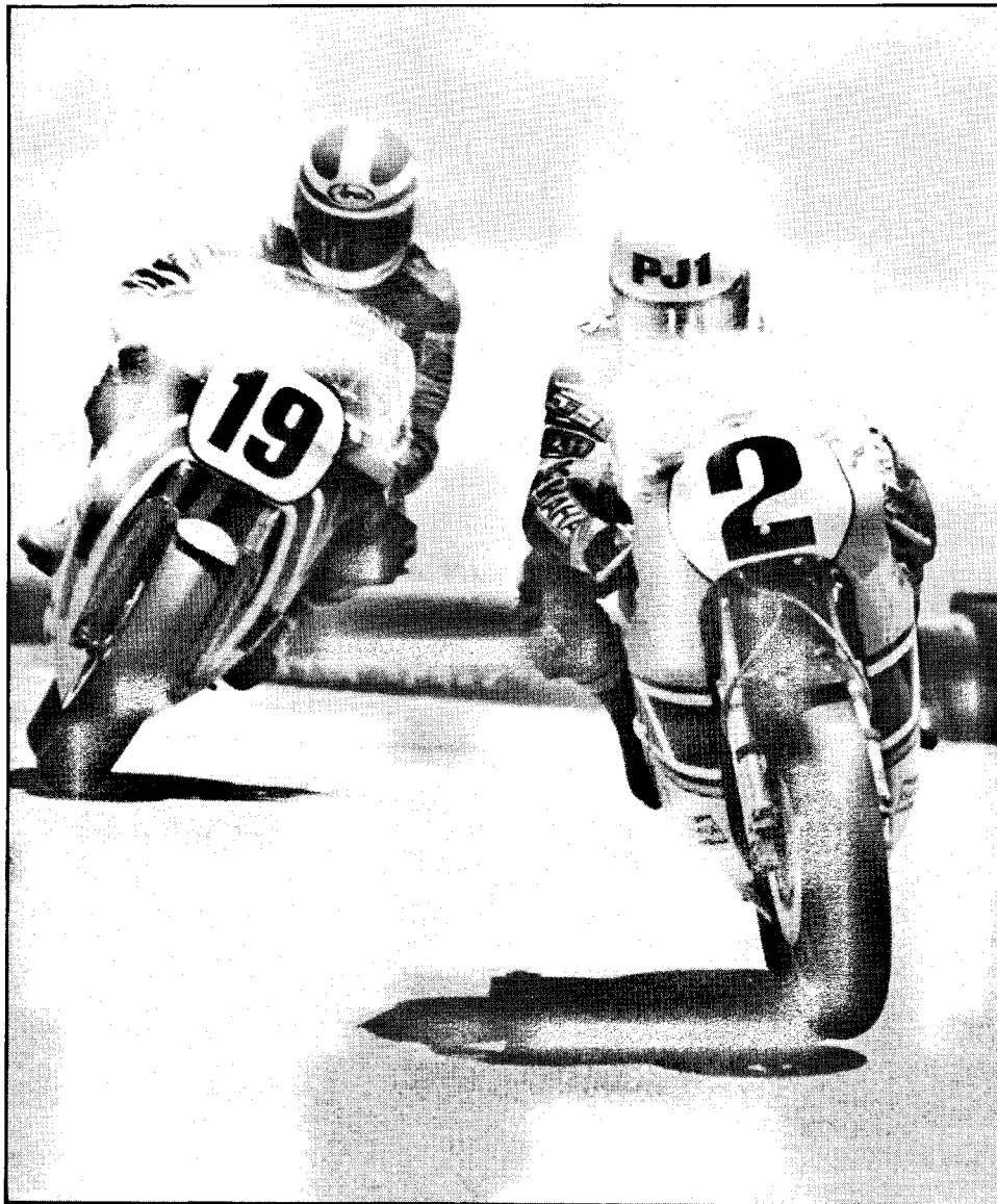
Kenny Roberts, the master of fast and precise steering, sets up for the right hander in the corkscrew. Notice the wheel sharply counter-steered to the left.
